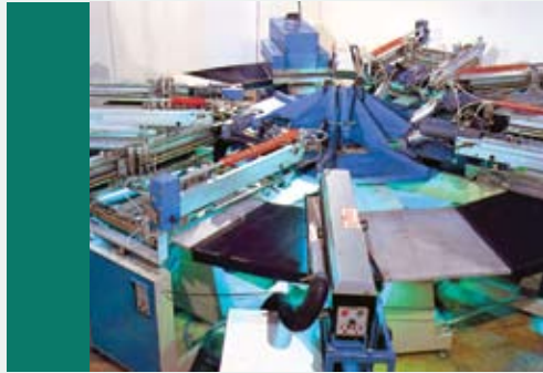
Hercules Horizon five-color carousel multi-printer with five built-in UV curing units
